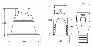
Note: MultiCyclone Support Stand is suitable for most Waterco Domestic Pool Pumps. Excluding Hydrostar & all Commercial Pumps.
