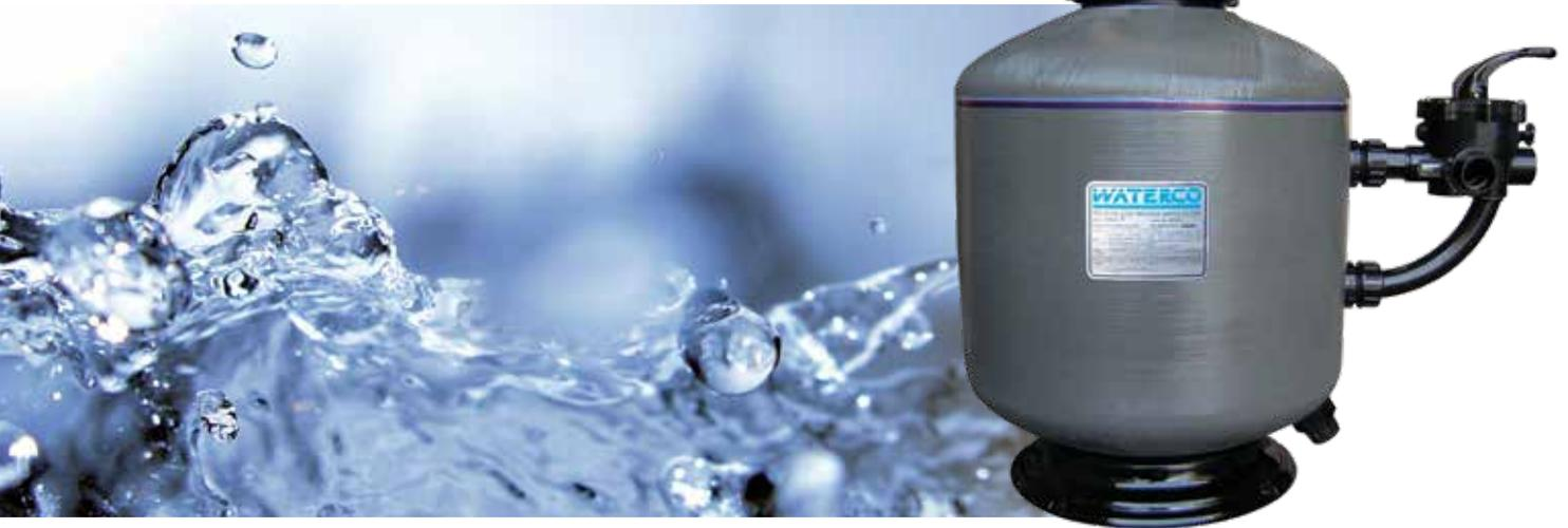
Waterco's digitally controlled filament winding machine faultlessly winds continuous strands of high quality fibreglass filament under controlled tension filament to create a seamless one-piece vessel with refined consistency and superior quality. There are no welds or seams or special tank linings which can corrode or electrolyse.
